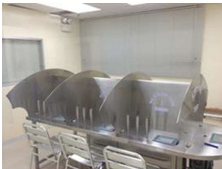
Figure 3: Olfactory Laboratory with Scentroid™ SS600 Olfactometer
